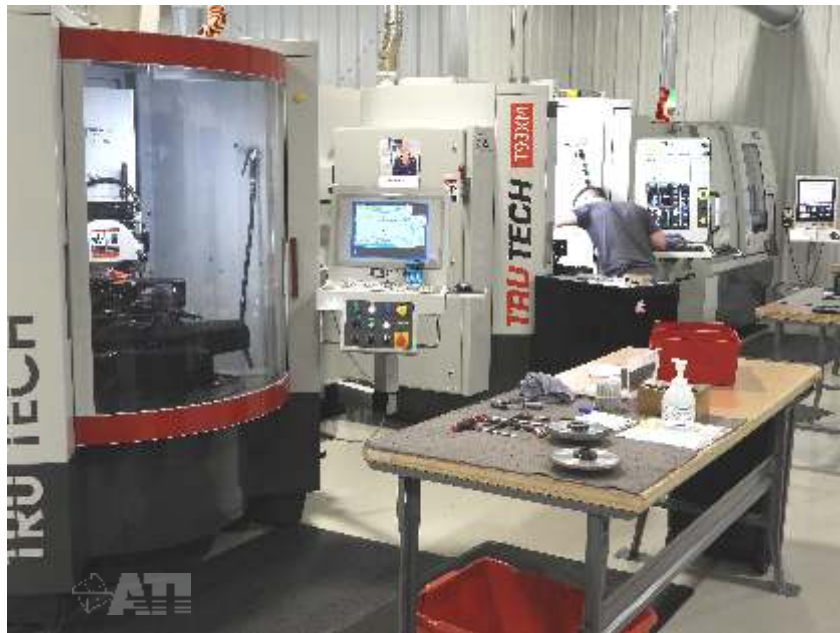
TRU TECH - Automated ultra precision profile grinding up to 3" diameter - sub micron accuracy of \pm .00005"
