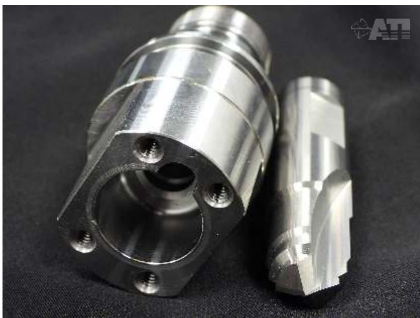
<< Custom step drill - keeping it rigid with stub flutes and straight flute geometry for more aggressive machining and reduced cycle times
